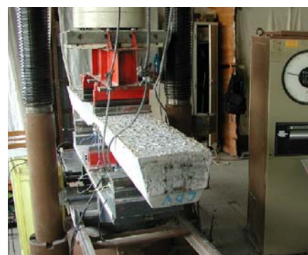
Fig. 4: Bending tension test
