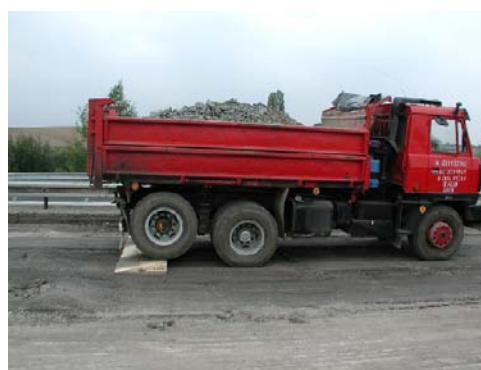
Fig. 7: Lorry travelling over the chock
