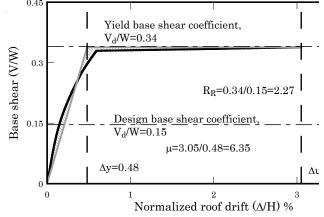
Figure 5. Idealized capacity curve of the MRFB
