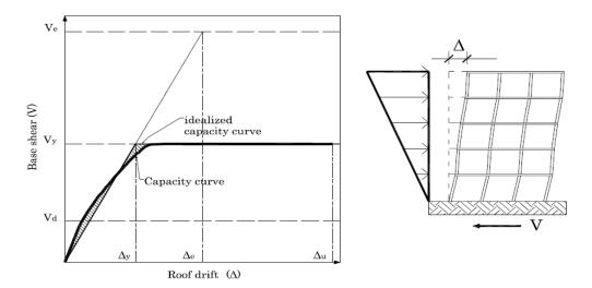
Figure 4. Scheme for determining the displacement ductility and the overstrength
