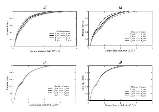
Figure 9. Evolution of the damage index of the a) 3 story, b) 6 story, c) 9 story and d) 12 story building
