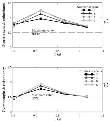
Figure 6. Overstrength and redundancy spectrum of the a) outer frames and b) inner frames
