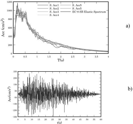
Figure 10. a) Sinthesized accelerogram b) EC-8 soil type B, elastic design spectrum and response spectra
