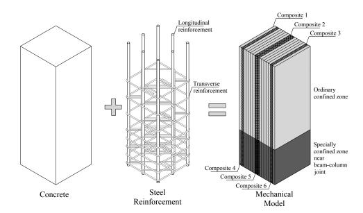
Figure 3. Discretization of the RC frame elements
