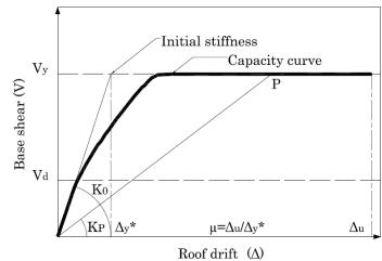
Figure 8. Parameters used in the calculation of the objective damage index
