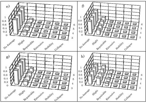
Figure 14. Damage probability matrices of a) outer and b) inner frames of 3 story buildings, c) outer and d) inner frames of 6story buildings, e) outer and f) inner frames of 9 story buildings and g) outer and h) inner frames of 12 story buildings
